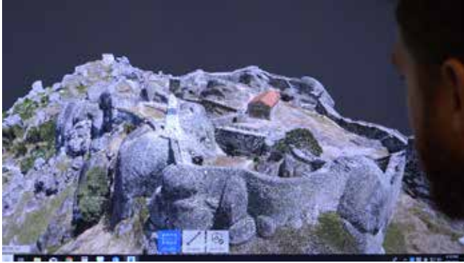
Edward Triplett examining a 3D point cloud of an historic Portuguese fortress.
